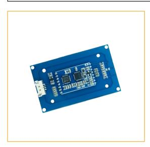
The **RFID Embedded HF Module Series R835** impresses with its integrated antenna. The R835 RFID Module is suitable for many applications within the medical sector, in vending machines for payment processing or also within the framework of access management. It is available with a **TTL interface** and in 4 different configurations: **DESFire, ISO 18000-3, PSAM, HF and MIFARE**.
