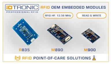
Our **RFID Embedded HF Modules M890** | **M900** | **R835** are suitable for a wide range of application within **RFID HF Frequency Areas**. The RFID HF Modules are applicable for about 100 transponder types from different ISO standards. They support **ISO 14443 A/B, ISO 15693, ISO 18000-3M3**
