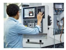
Machines in large productions for plants require authorized access. The integration of the M890 module into the control panel of a machine protects the machine control against unauthorized access. The responsible employee logs into the panel using his RFID tag. The control panel then releases the control elements and the employee can operate the machine.
