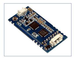
The Integration of an RFID OEM Module in diagnostic systems validly identifies the batch packaging of the respective test. RFID OEM Module M890 operates in the high frequency range of 13.56 MHz and validly reads out all data in the close range of up to 8 cm. After successful tag authentication, all test parameters are stored in the system. The pre-defined test parameters and all patient data can be written to the RFID OEM module. This enables the transfer
